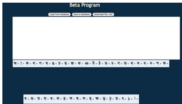
Figure 1: The top-level menu items for character entry. The 11 vowels are represented by the first menu item in the top row. The second item in the top row represents the medial diacritic representations of the eleven vowels. The last three items on the bottom row represent special characters, numerals and punctuation, respectively.
