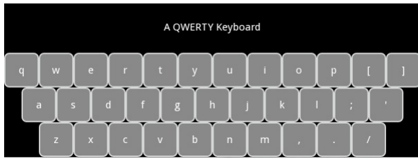
Fig. 6. A simple, abstracted example of a keyboard interface designed in the KIVY UI framework.
