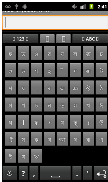
Fig. 14. This Assamese keyboard was implemented as an AnySoftKeyboard plug-in. It was designed by the genetic algorithm after 50 generations. The diacritics are placed in a pop-up menu.
