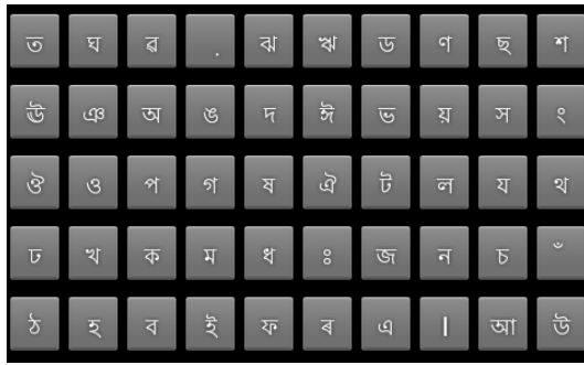
Fig. 18. Android keyboard designed for two finger input. This keyboard has a lower bound of text input estimated to be 22.6 WPM.
