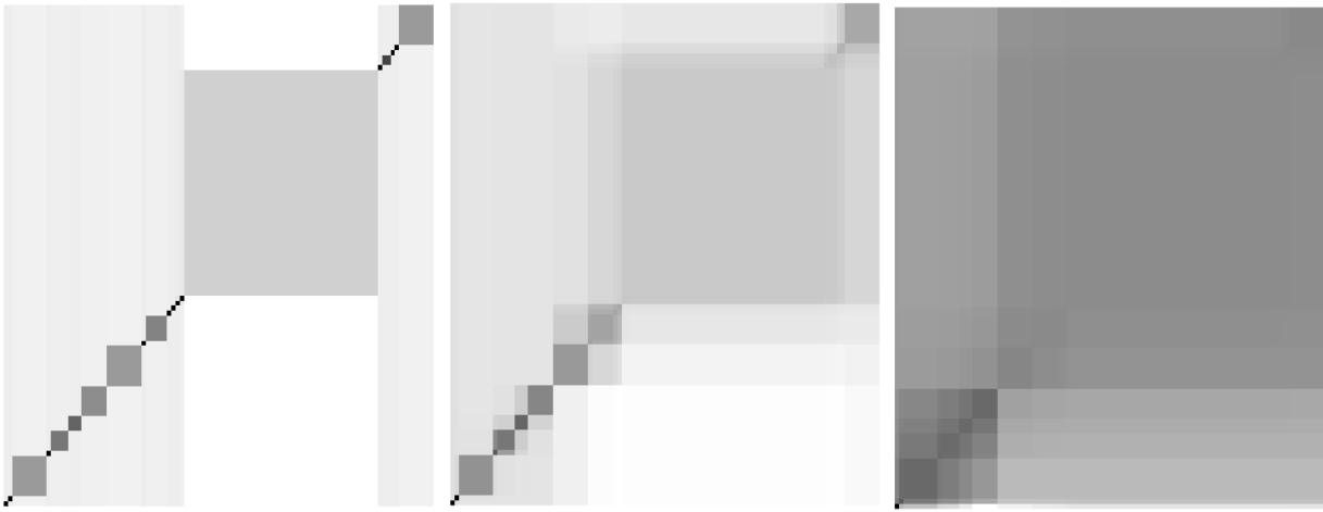
Fig. 1. Similarity matrices at varying K displayed as heat maps, darker representing more similar entries. Similarities scores calculated with higher values of K correspond to broader time scales (months vs. days). Left to right, K is increased by a factor of 10 at each iteration.
