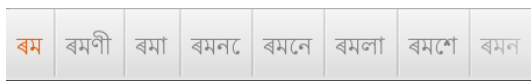
Fig. 16. The word prediction menu. This menu appears after at least two characters have been entered.
