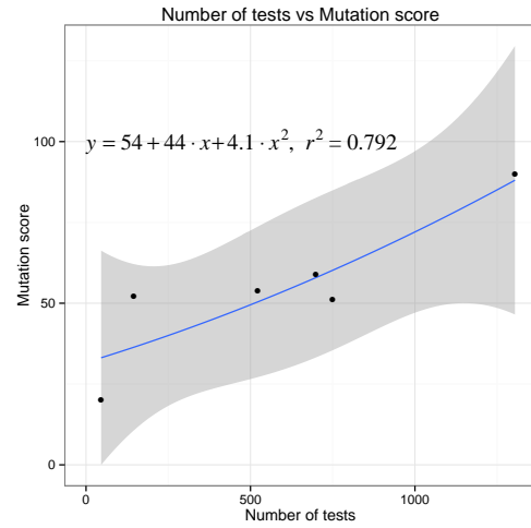
Figure 9: Number of tests compared to mutation score for applications with >500 tests
