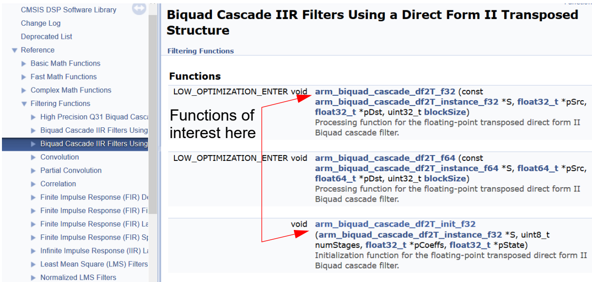
Figure 14: CMSIS-DSP IIR cascade of second-order sections float32_t filter detail.
