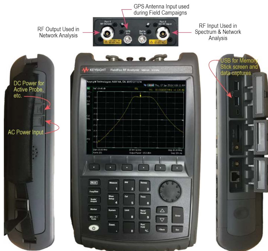
Figure 14: The Keysight N9914A spectrum/network analyzer, showing the front panel and side and top connections.
